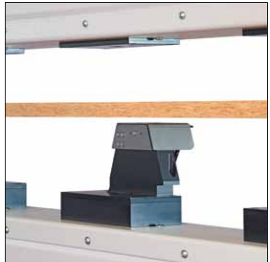
Laser thickness measurement of a wood based panel
