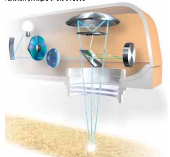
Function principle of the IR 5000
